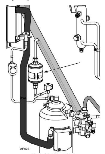
Figure 68: Filter Drier
