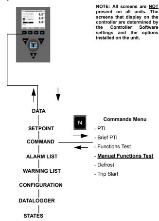
**Figure 27: Manual Function Test**
