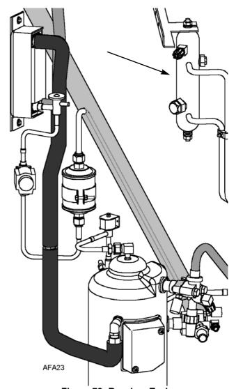
Figure 72: Receiver Tank
