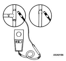
Figure 62: Test for Refrigerant Leaks
