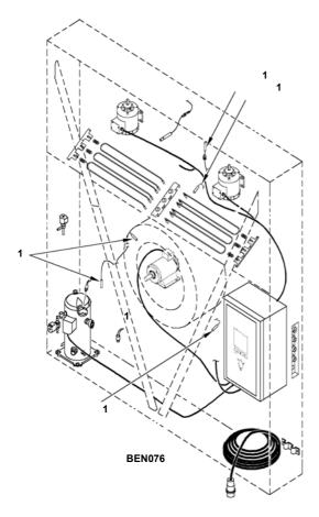
Figure 47: Temperature Sensors
