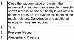
Figure 66: Pressure Rise Levels Off After Evacuation Indicates Moisture in System
