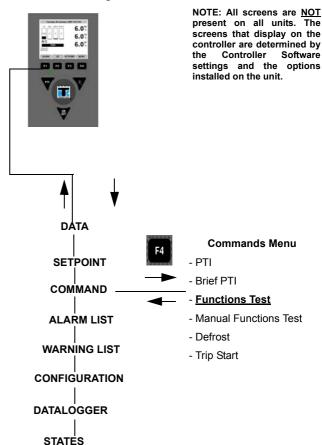
Figure 26: Function Test
