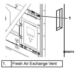
Figure 7: Fresh Air Exchange Vent
