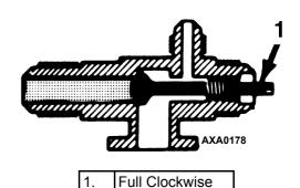
Figure 54: Service Valve Front Seated
