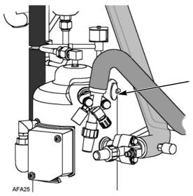
Figure 46: Compressor Discharge Temperature Sensor
