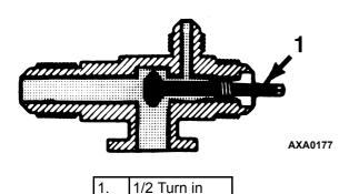
Figure 53: Service Valve Open to Port
