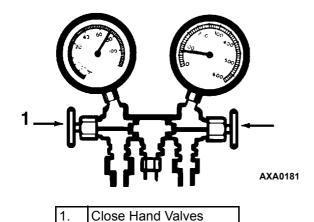
Figure 57: Gauge Manifold Closed to Center Port
