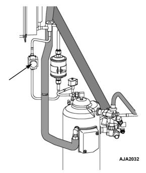
Figure 74: Vapor Injection Valve
