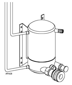
Figure 73: Water-Cooled Condenser Tank
