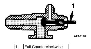
Figure 52: Service Valve Back Seated
